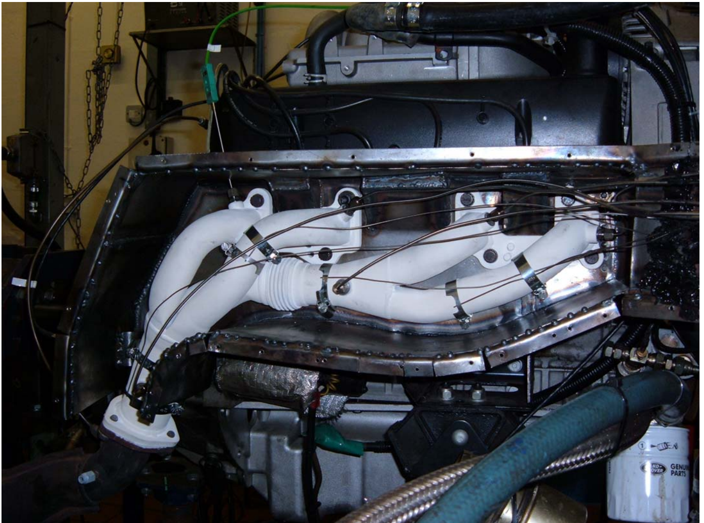
Figure 2– Zircotec Coated Manifold Prior to Test
