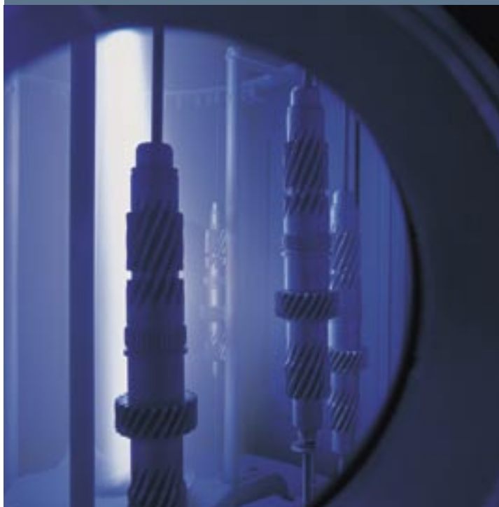
A column of ions is created in the centre of the chamber and attracted towards the components, to etch them prior to PVD or PACVD coating
